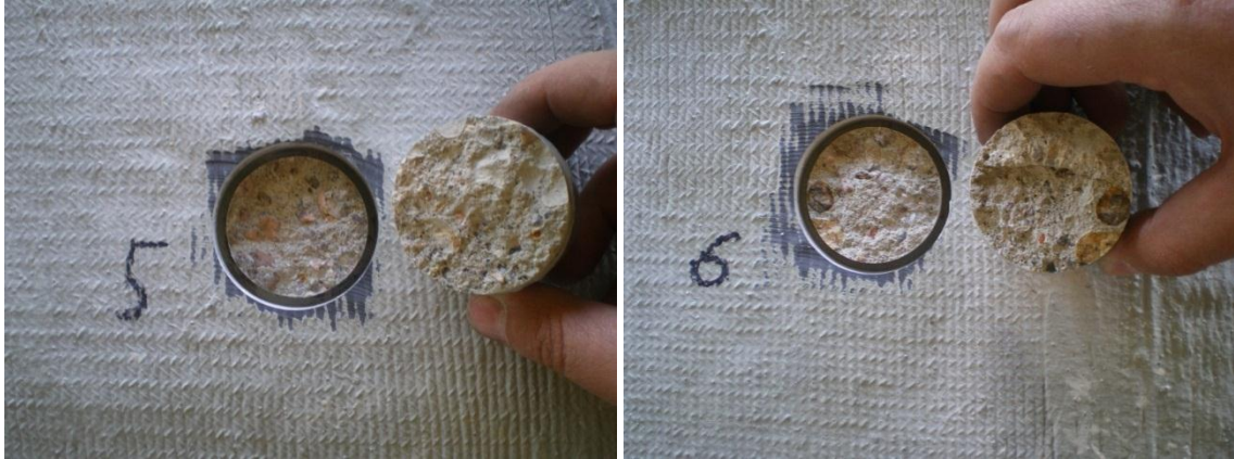
Figures B20 and B21. Test No.23, weak bond strength (poorly mixed concrete?), and Test No.24
