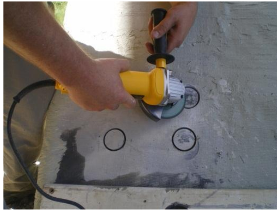
Figure 3.30. Removing the acrylic paint later before adhering the aluminum pucks
