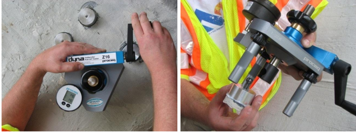
Figures 3.38 and 3.39. Conducting a pull-off test with the digital manometer reading and removing the tested puck from the pull-off tester
