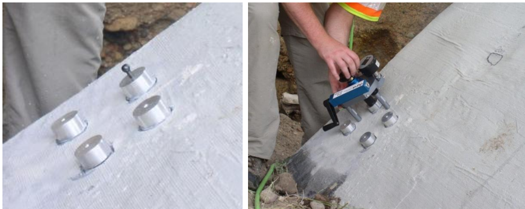
Figures 3.36 and 3.37. Spherical headed bolt threaded into puck and placing the pull-off tester to engage the spherical headed bolt
