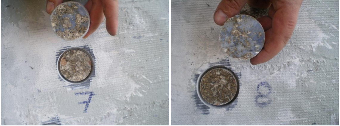
Figures B6 and B7. Test No.7 and Test No.8, weak bond strength
